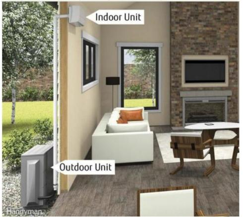
Thin copper tubing is used to pump refrigerant from the outdoor compressor directly into an indoor air-handling unit, where the air is quinetly distributed to the interior space. This eliminates the need for basement or attic evaporators and bulky, expensive ductwork. Mini splits are easy to install and usually require only a 3- to 4-inch hole through a wall or ceiling to connect the indoor and outdoor units.
