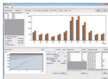
Energy saving graph data: This graph compares the electricity consumption with the previous month and previous year to make it easy to analyze the energy saving effect.
