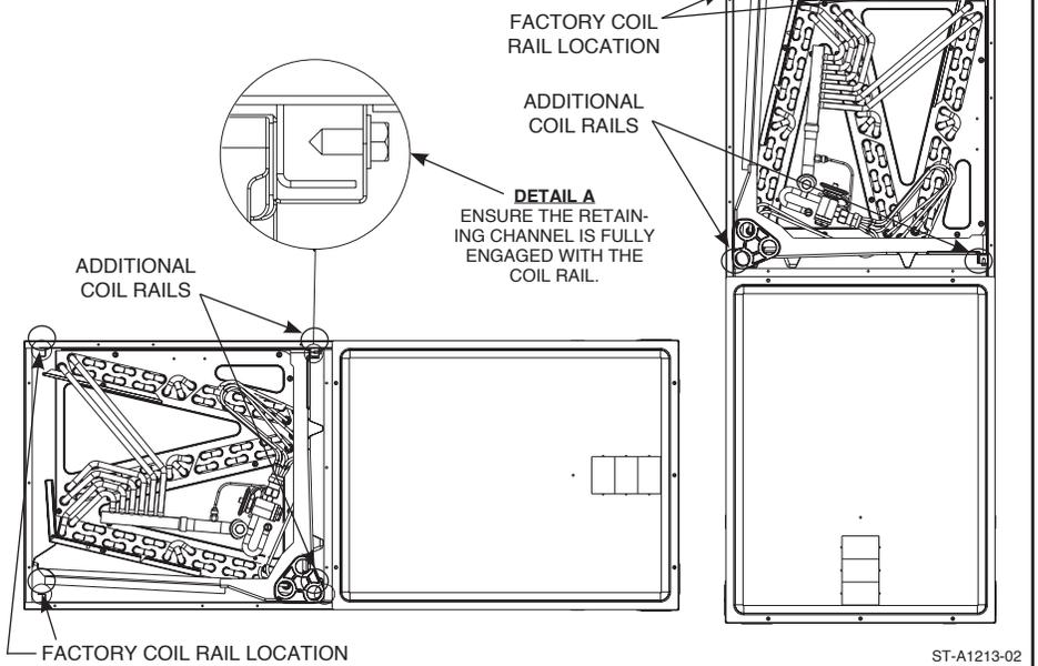
**FIGURE 7****INDOOR COIL AND DRAIN PAN DETAILS**
