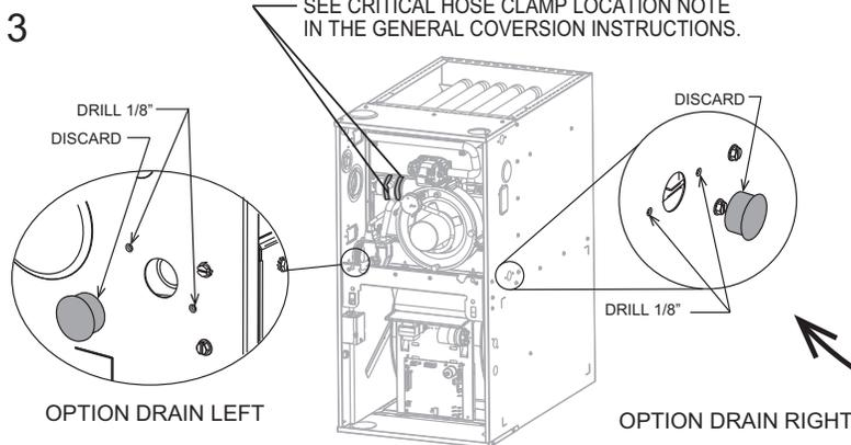
DETERMINE RIGHT OR LEFT DRAIN OPTION. LOCATE 7/8" HOLE IN JACKET SIDE. REMOVE PLUG - DISCARD. DRILL (2)  $\phi$ 1/8" HOLES FOR THE BULKHEAD COUPLING.
