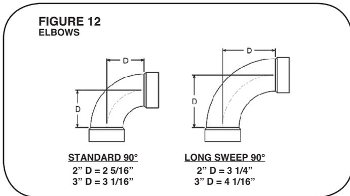
A long-sweep (AKA Long-Radius) 90° (1/4 turn) elbow has an equivalent vent length of 5 feet of straight pipe for either 2 inch or 3 inch plastic pipe. A standard 90° elbow has an equivalent vent length of 10 feet of straight pipe. This equivalent length can be used in circumstances where it might be necessary to lengthen the vent at the outside of the structure, such as in areas with large accumulations of snow in winter. **Table 3** shows the equivalent lengths of different types of elbows.
