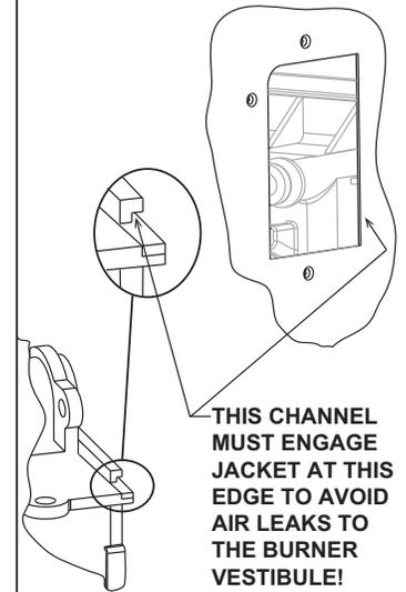
**THIS CHANNEL MUST ENGAGE JACKET AT THIS EDGE TO AVOID AIR LEAKS TO THE BURNER VESTIBULE!**
