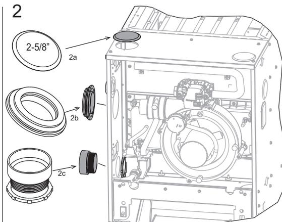
NOTE: IF THE IDB COUPLING IS REMOVED, IT MUST BE REPLACED IN THE PROPER ORIENTATION. AN ARROW IS PRESENT ON THE COUPLING TO INDICATE THE DIRECTION OF EXHAUST FLOW. MAKE SURE THE ARROW POINTS IN THE CORRECT DIRECTION.
