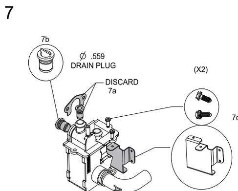
7a - REMOVE THE SMALL MOUNTING BRACKET AND THE .403" DRAIN PLUG - DISCARD.
