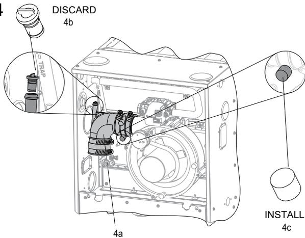
4a - RE-INSTALL ELBOW AND COUPLINGS (FROM STEP 1) IN THE ORIENTATION AS SHOWN.
