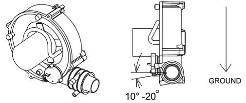
ROTATE INDUCER COUPLING TO ENSURE DOWNWARD FLOW OF CONDENSATE FROM FLUE VENTING
