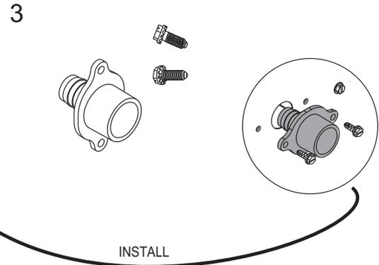
INSTALL BULKHEAD COUPLING USING (2) SCREWS.
