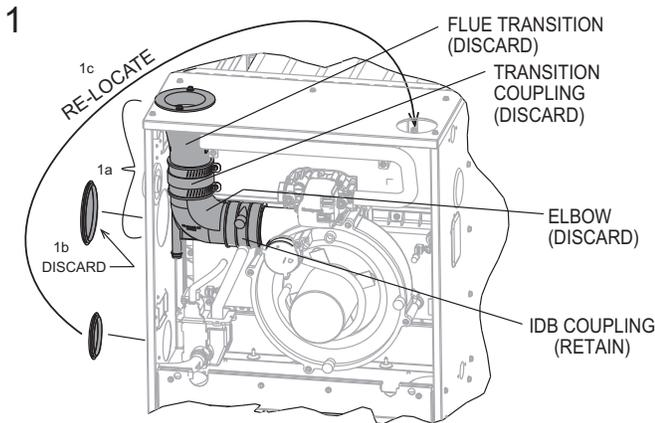
1a - REMOVE FLUE TRANSITION, TRANSITION COUPLING, AND ELBOW. **(NOTE: REMOVE INDUCER COUPLING W/ELBOW FOR EASIER REMOVAL).**
