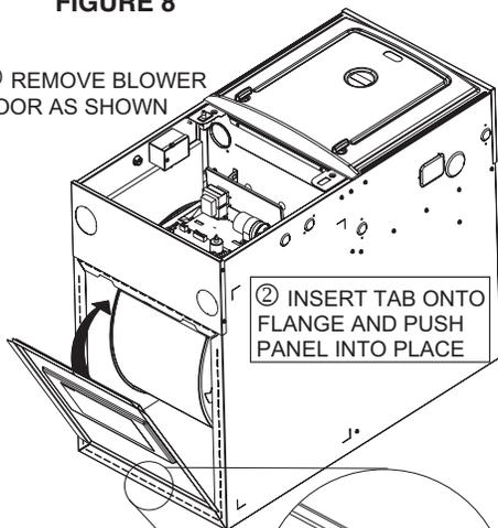
② INSERT TAB ONTO FLANGE AND PUSH PANEL INTO PLACE
