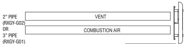
MAINTAIN 12" / 31cm FOR THE U.S. AS THE MINIMUM CLEARANCE ABOVE THE HIGHEST ANTICIPATED SNOW LEVEL OR GRADE WHICHEVER IS GREATER. IN CANADA TERMINATIONS MUST CONFORM TO CSA B149.1-10, SECT. 8.14.
