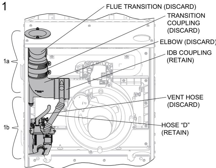
1a - REMOVE FLUE TRANSITION, TRANSITION COUPLING, AND ELBOW.
