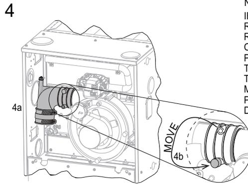
4a - RE-INSTALL ELBOW AND COUPLINGS (REMOVED IN STEP 1) IN THE ORIENTATION AS SHOWN.
