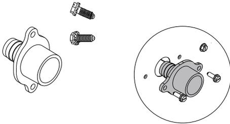
INSTALL BULKHEAD COUPLING USING (2) SCREWS.
