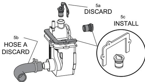
**NOTE: TO PREVENT DAMAGE TO THE TRAP, THE INSTALLER MAY ELECT TO INSTALL IT DURING A LATER STEP. (AFTER THE UNIT IS ROTATED)**
